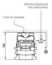
The extinguishing chamber cover is part of the standard scope of delivery for the C360A/150, C360A/300 and C360A/500 series.
