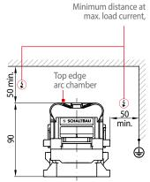
i It is permissible to use the C360A/150, C360A/300 and C360A/500 series without arc chamber cover, taking into account additional clearance dimensions.
