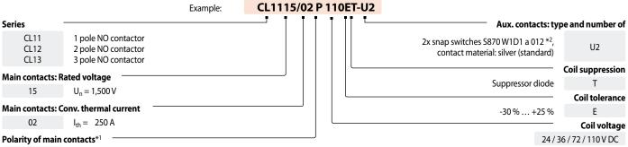
P DC with blowout and arc chute with brass baffels (with 2 and 3 pole versions: for parallel connection)
