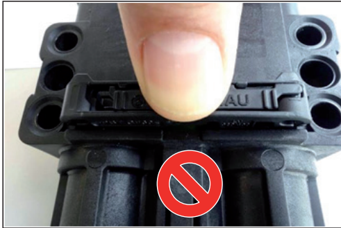
Fig. 21: Do not push in the slider in the locked condition and not with a centric application of force.
