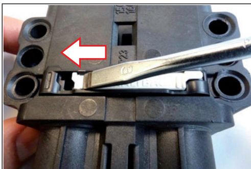
Fig. 23: Push the slider with a slotted screwdriver by approx. 4 to 5 mm up to the end stop into the locked position so that recess and crossbar are overlapping.
