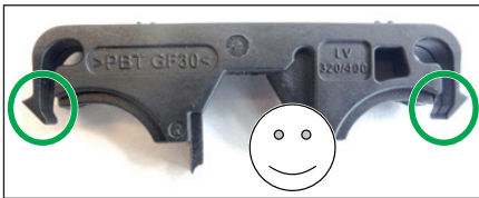
Fig. 55: LV 320/400 S slider with latching hooks that are intact
