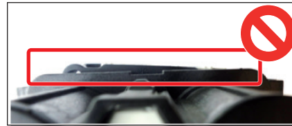
Fig. 52: Slider not parallel to the housing and thus not in the correct position. Left side of the slider is not latched.
