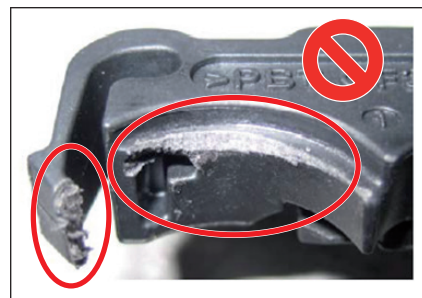
Fig. 54: Two latching hooks are broken. The slider is not o.k. as soon as one of the four latching hooks is missing or is broken or if the bearing surface is damaged.
