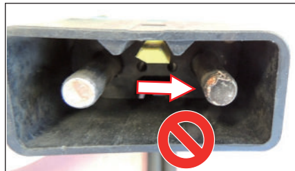
Fig. 43: Right contact with material covering or removal on pin contact
