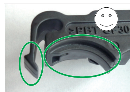
Fig. 53: All latching hooks (2 items per half) are o.k. ! Only one half is illustrated here.
