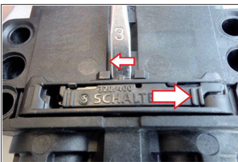
Fig. 28: Move the lock into the unlocked position up to the end stop. Carefully lift the slider with a rotary movement.
