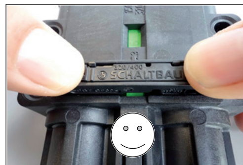
Fig. 20: Push in on both sides the slider in the unlocked condition with an application of force on both sides (for the fastening of the main contacts) until it latches.
