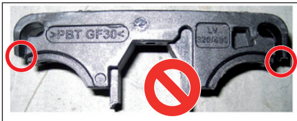
Fig. 56: LV 320/400 S slider with damaged latching hooks
