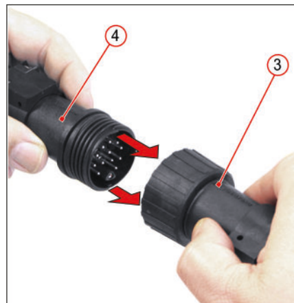
Fig. 28: Slide off plug (3) from receptacle (4)
