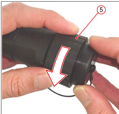
Fig. 30: Screw down union nut (5) hand-tight
